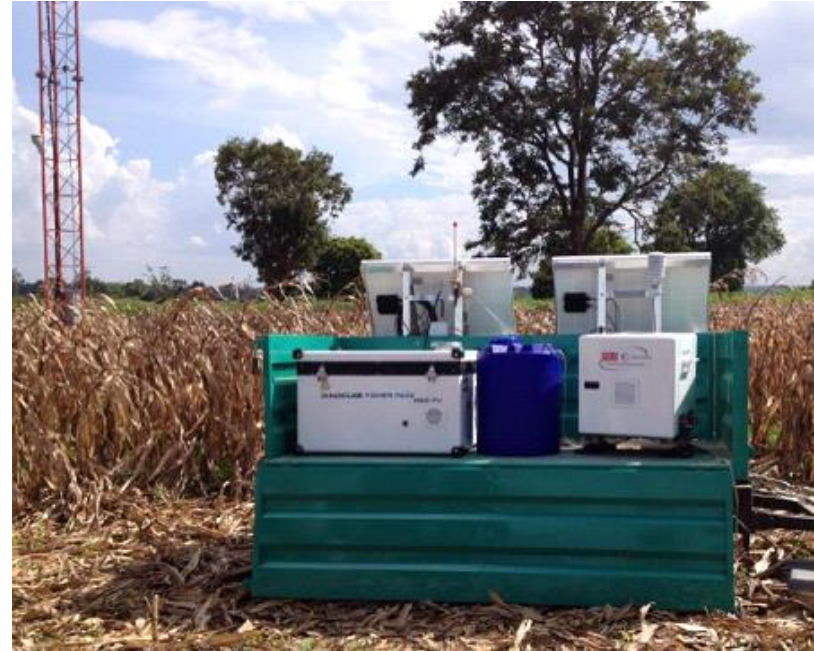
WINDCUBE v2 and POWER PACK in a trailer (courtesy of WIND ENERGY HOLDING - THAILAND)
