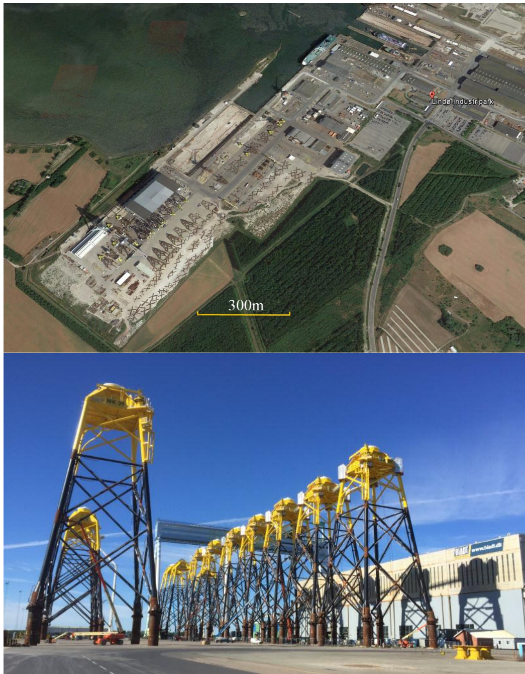
Figure 3.1 Port of Odense (Lindø Industrial Park, upper, Google earth, 2015) and 600t jackets ready for load-out (lower)
