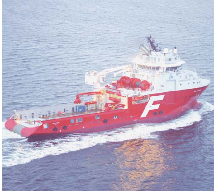
Far Sapphire is a UT732 AHTS owned by Farstad Shipping, equipped with an energy-efficient hybrid propulsion system.
